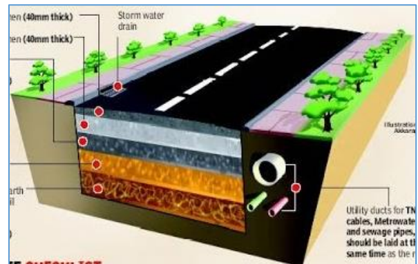
Figure No 6.14: Typical Conceptual Plan of Road Side Drainage
