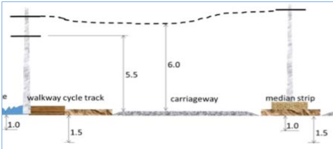
Figure No 6.12: Electricity lines and Cable Poles
